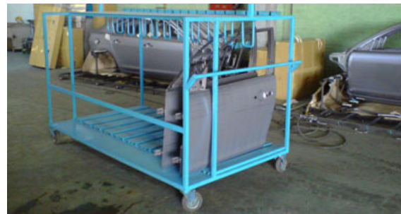
Fig. 1. Mobile material handling shelf
